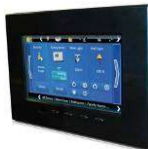
Embedded Automation – mPanel (Digital Home Device) ARM architecture-based – Marvel XScale
